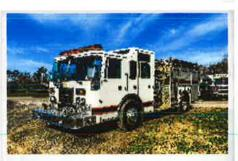
Waterous 1250 GPM Pump, 1000 Gallon Tank, Detroit Diesel
