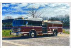
Waterous 1500 GPM Pump, 500 Gallon Tank, Cummins Diesel
