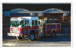
le 1500 GPM Pump, 750 Gallon Tank, Cummins Diesel, Foam....
