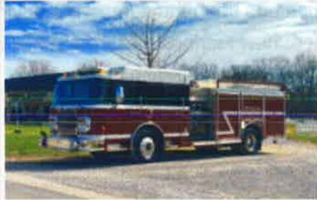
Waterous 1500 GPM Pump, 500 Gallon Tank, Cummins Diesel
